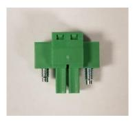
Attach the power converter with the 2-pin terminal block to the green adapter you removed and plug in the supplied power adapter 12VDC 1.2A into the other end of the converter. Then re-insert the green adapter into the device.
