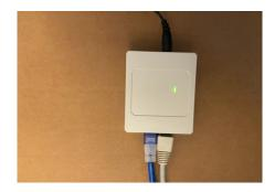
Be sure to attach the enclosed power cord to the PO injector.
