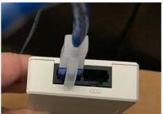
Attach the enclosed wire in the port to the right of the Greenpacket's PO injector. The other end connects to the router.
